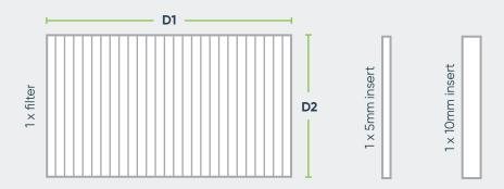
$\textbf{NOTE:} \ \text{The inserts are specially designed to slide into the filter profile at } \textbf{D2} \ \text{side}$
