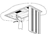
15. Install return air filters and/or fresh air filters. Ensure the filters are installed with the recess part of the filter facing down.
