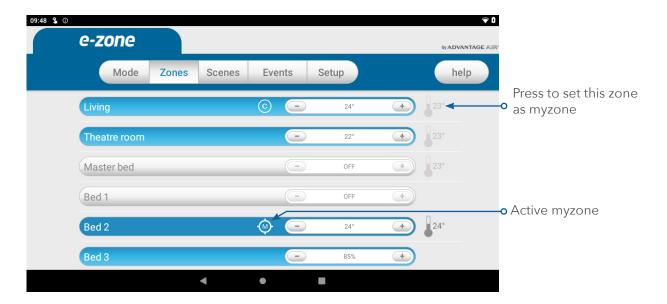
This feature can be particularly important when you have an unusually high requirement for air conditioning in a particular area. For example, a group of people watching a movie in Theatre room with all the electronic A/V equipment turned on will have a larger requirement for air conditioning than in other rooms in the house. Setting the Theatre as myzone will ensure that the system continues running until the temperature set-point for that room is achieved.
