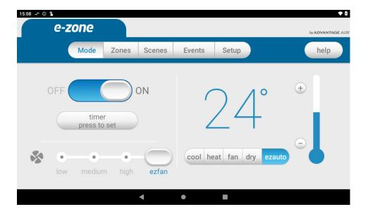
This feature is ideal for ever-changing weather conditions, during the day and night. e-zone will change the mode to heat on a chilly morning and to cool during a hot midday. Like in eztemp, it will automatically assign the myzone to an open zone that needs a higher requirement.
