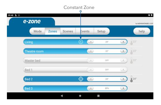
In this example this zone may open automatically to relieve excess air pressure when needed.
